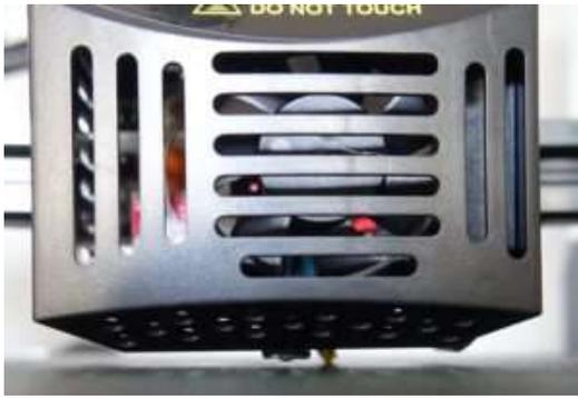
I had to loosen the two fastening screws in order to push the housing up as much as possible in the seat, so that the LED keeps a reasonable flight height and does not fly too close to the component. In the photo, the housing is at the top stop, which makes it narrow at the top for the safety clips on the Bowden's push-fit.
