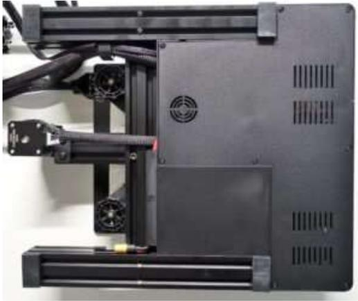
Both carriages and all motor mounts are made of thick sheet metal, typical of V-slot printers.
