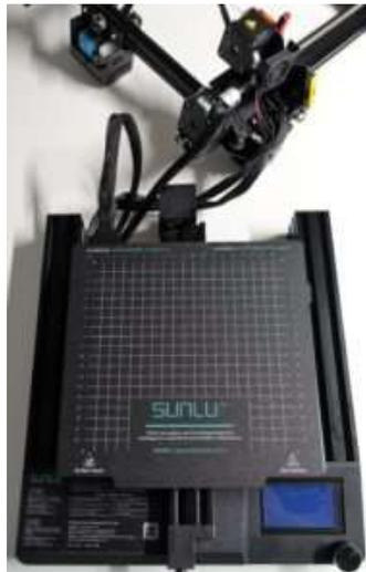
The finished wiring connecting the two components requires some care when assembling. All plug connections are secured with hot glue at the factory so that nothing can come loose during transport and operation.
