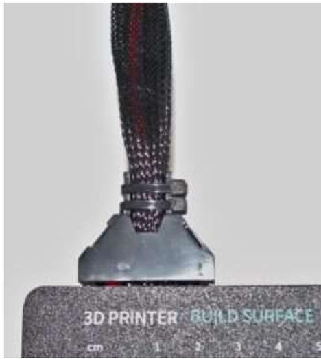
The pressure mat is a relatively firm, rough plastic mat. Its surface survived the test prints without leaving any traces. The printed parts have a low residual adhesion after printing and cooling. That's fine. But the residual adhesion is not enough to hold the printed part in place after the filament has run out or a power failure to cool down and restart printing. As a magnetic mat, it is easily exchangeable and you can put on an Ender 3 mat of your choice.
