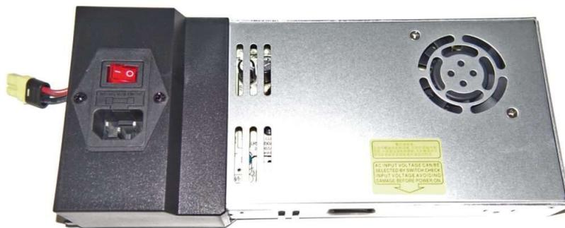
The power pack is screwed precisely and stably to a module with an injection-moulded housing for the power socket and switch, so that no 230V lines are exposed. It is screwed directly to the right Z-pillar with two screws. The entire power is delivered to the mainboard via the XC connector.
